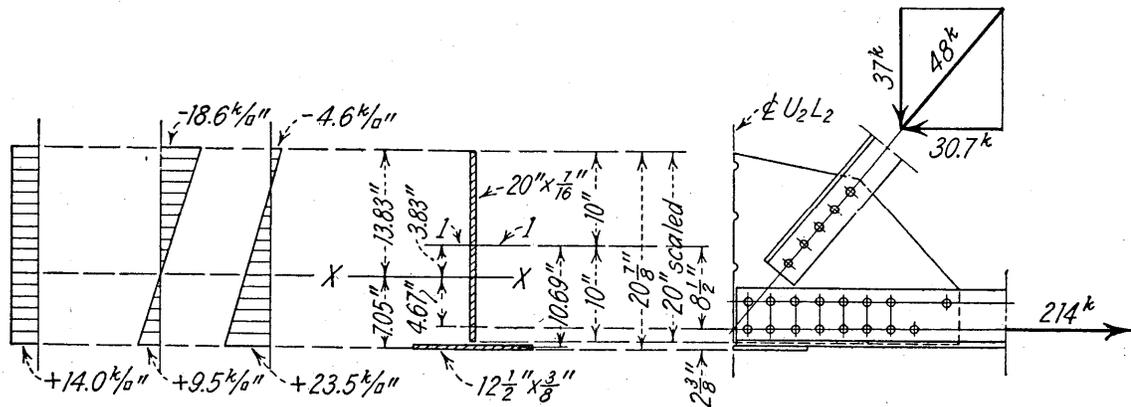
Fig. 9. Calculated stress distribution in a gusset plate (Shedd, 1934).
