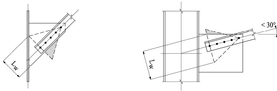
Fig. 7. Cases where the Whitmore width is only partially effective.
