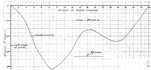
e. Shear stress at section B-B
