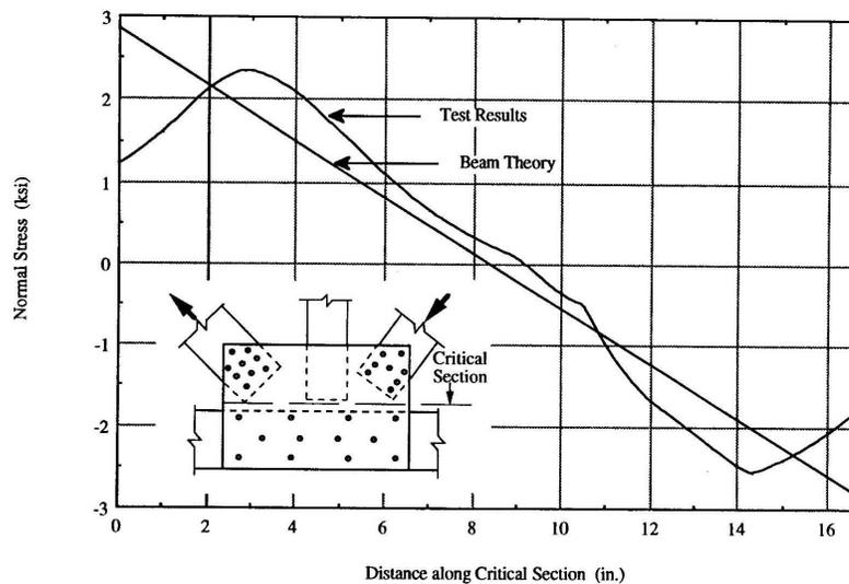
Fig. 11. Bending stress by Whitmore (as re-drawn by Yam and Cheng, 1993).
