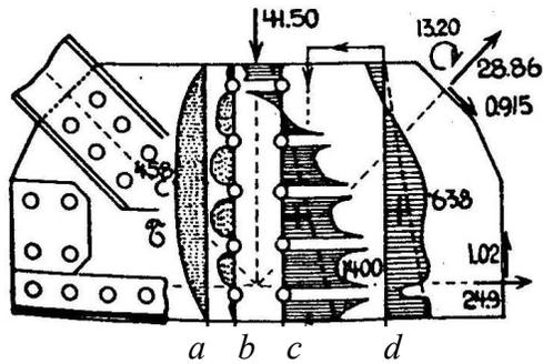
Fig. 8. Normal and shear stresses by Wyss (1923).
