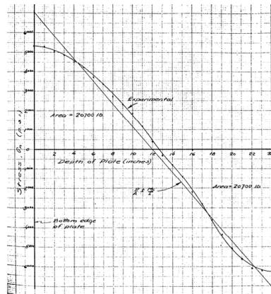
b. Normal stress at section A-A
