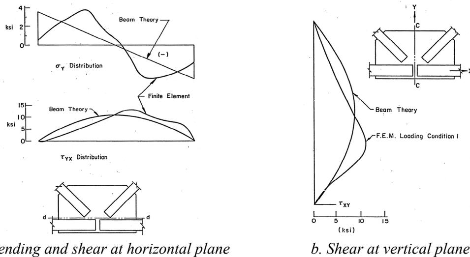
Fig. 13. Bending and shear stresses from Struik (1972).
