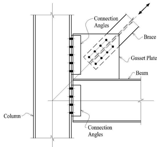
*Fig. 1. Vertical brace connection.*
