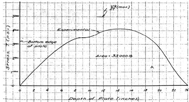
c. Shear stress at section A-A
