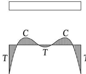
*Fig. 16. Residual stress pattern for a plate with flame-cut edges.*
