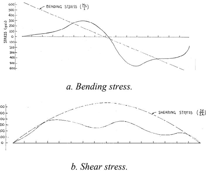
Fig. 10. Bending and shear stresses by Sandel (1950).
