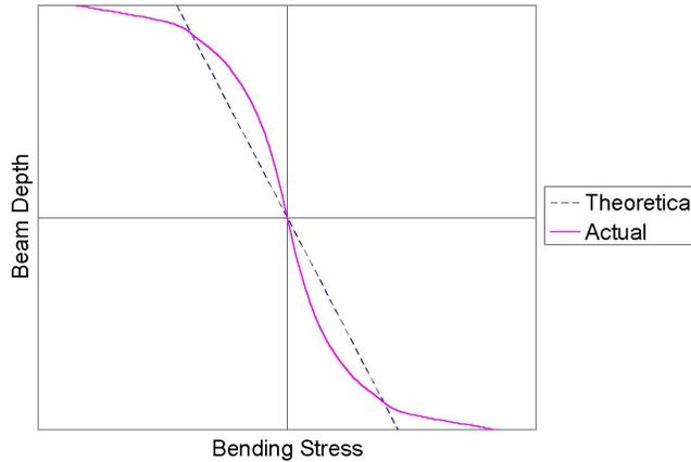
*Fig. 15. Bending stress in a deep beam with a length-to depth ratio of 1.0.*
