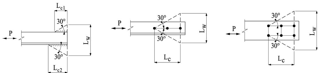
Fig. 6. Effective width for various connection configurations.
