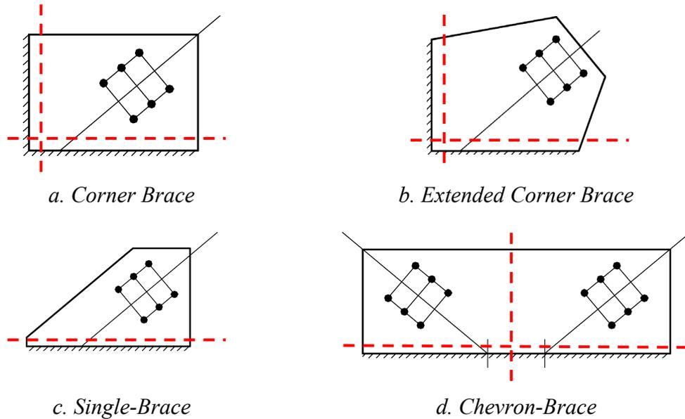
Fig. 14. Location of critical section.
