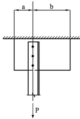
Fig. 18. Gusset plate connection with axial load and moment.
