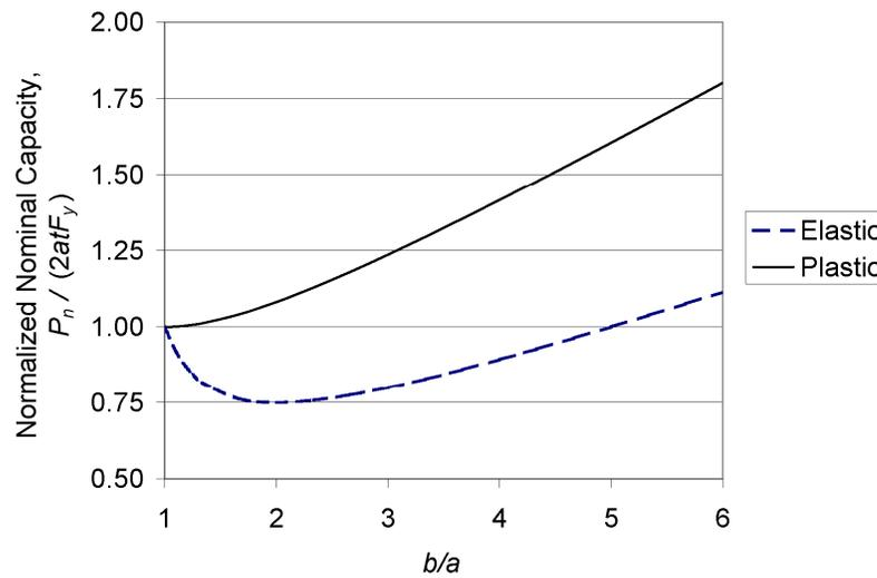
Fig. 19. Elastic versus plastic design for gusset plates with axial load and moment.
