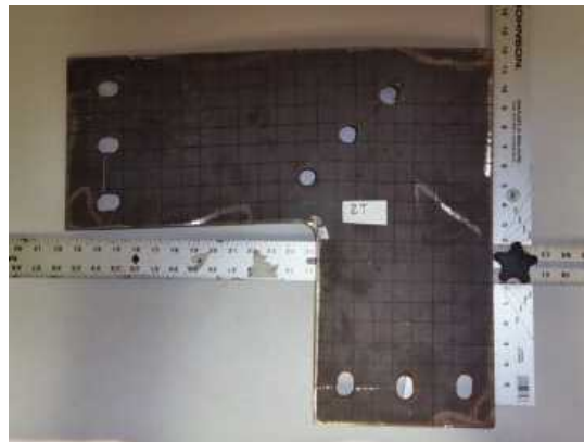
Figure 7. In-plane deformation of Specimen 2T.
